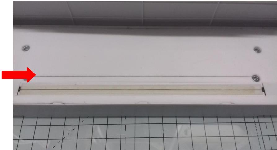
I drew a pencil line about 1cm (approx.  $\frac{1}{2}$ " ) above the heating wire & used that as a guide for lining up the edge of the pouch; as you can see indicated by the red arrow in the picture to the left.
