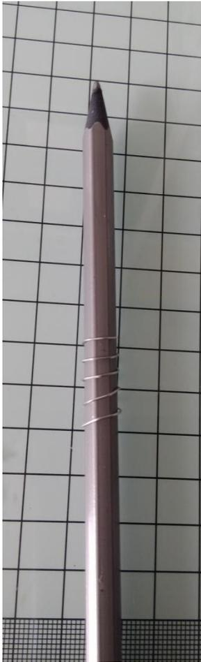
Now you need to wrap your wire around the pencil to form the springs, bearing in mind you want the spring to compress in order to fit into an envelope I recommend that you only wrap the wire four times around the pencil & then trim it off. One coil at each end will be used in the construction leaving you three remaining coils for the bounce affect.
